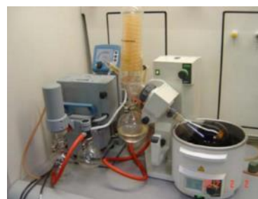
Evaporation of solvents ( p = 25\text{ mbar} , T = 55\text{ °C} )
