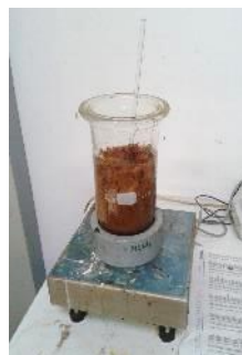
Mixture of wood, EG, H_2SO_4 in reactor
