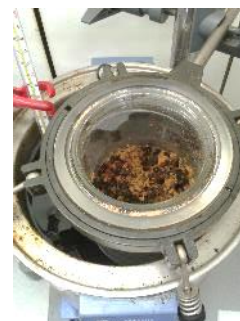
Reactor in oil bath ( T = 180\text{ °C} )
