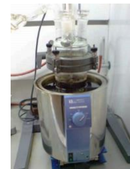
Heating and stirring ( T = 180\text{ °C} , t = 90\text{ min} )
